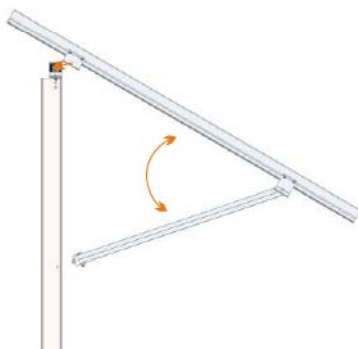
Step 3: Install the Assembly of Beam
